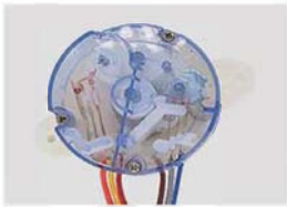
MODEL NO. DXTSF15-6 TIME 15min TYPE 6 Wires
